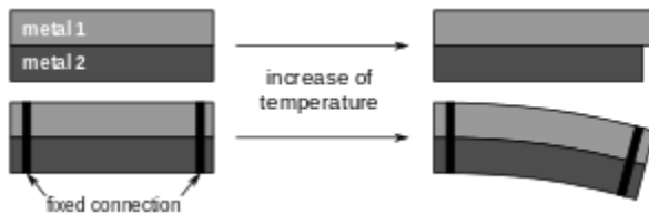
Figure 2. Bimetallic strip diagram showing
